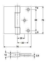
Matt finished stainless steel 316 (1.4401) with flat end caps. Stainless steel pin diameter 7 mm. With stainless steel washers and 3 countersunk holes for M5 screws. One leaf without holes
