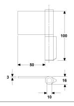
Stainless steel 316 (1.4401) Lift-off hinge with stainless steel pin dia. 10 mm. Flat head with flat hinge leaf and one s/s washer. Without holes. Hinges are handed.
