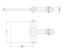
Stainless steel 316 (1.4401) cast hinge with fixed pin with beveled edge. 4 knuckles with 4 countersunk holes for M8 screws.
