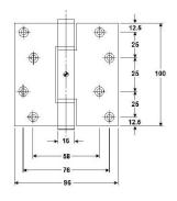
Matt finished stainless steel 316 (1.4401) with flat end caps. Stainless steel pin diameter 10 mm. With stainless steel washers and 8 countersunk holes for M5 screws. Suitable for recessed and flush surface situation. Suitable for extra large openings; for example, wheelchair access.
