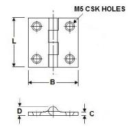
Mirror polished stainless steel 316 (1.4401) body with stainless steel pin. Flat back hinge with 4 knuckles and with 4 countersunk holes for M5 screws.
