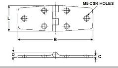
Stainless steel 316 (1.4401) body with fixed stainless steel pin. 6 knuckles. Flat back hinge with 6 countersunk holes for M5 screws.
