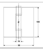
Stainless steel 316 (1.4401) body with flat end caps and removable stainless steel 316 pin and 2 washers. One leaf flat back and one leave swaged, without holes.
