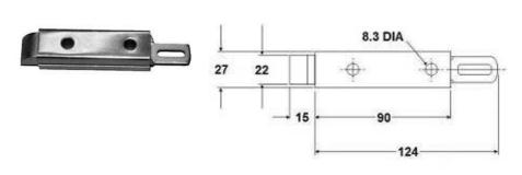
Code no. 98-3306 END SLAM L 90/124mm Material: zinc galvanized Fitted with release lever
