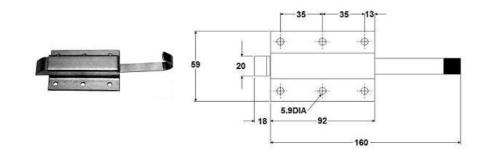
Code no. 98-3301 END SLAM L 92/160mm Material: zinc galvanized Fitted with release lever
